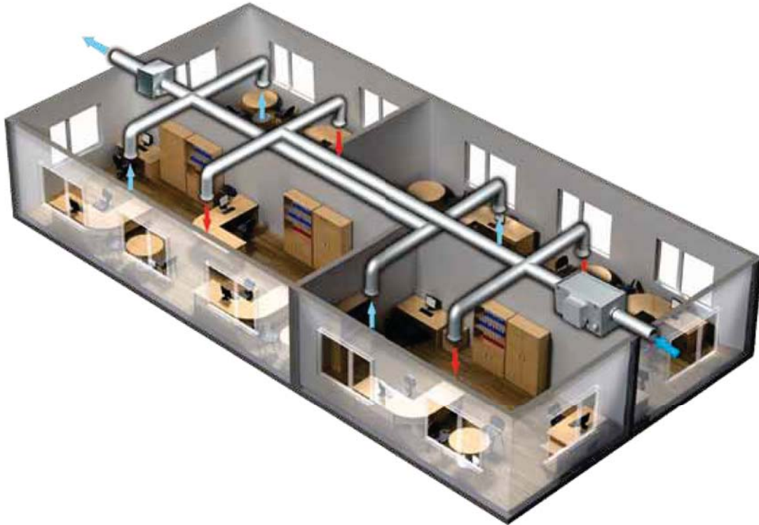
MPA unit office air exchange example.
