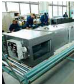
Air handling units workshop
