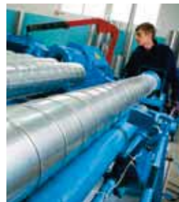
Spiral wound ducts workshop
