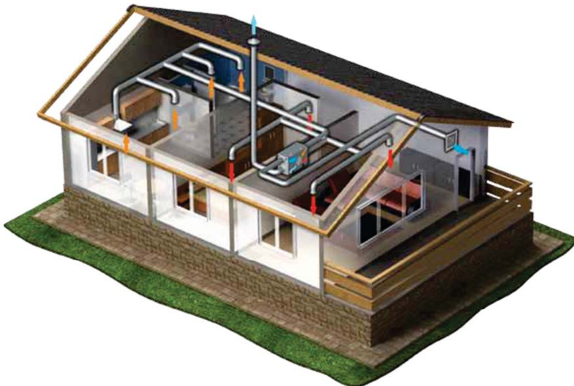
VUT EH EC ventilation and air exchange example in the cottage.
